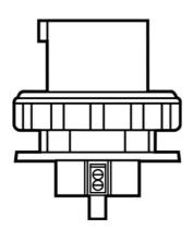
Triple-Pole, 4-Wire, Pin and Sleeve Inlet. 100A, 3/600V.
