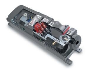
Triple pole, Four wire, Fusible Mechanical Interlock Receptacle. 6 amp, 3 Phase 600V. 15 HP Standard to 40 HP Max
