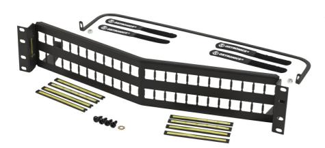
48 port unloaded angled panel for rear loading HDJ series of jacks and accessories. Includes rear management bar and straps. Occupies 2 rack units of space, 3.5" x 19".
