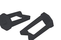
Cable retention ring kit consists of 4 rings to improve cable management from the overhead pathway racks. The rings have a quarter turn feature which makes them easy to install, even after the rack has been deployed. The rings can mount to the front surface as well as the side surfaces of the rack.
