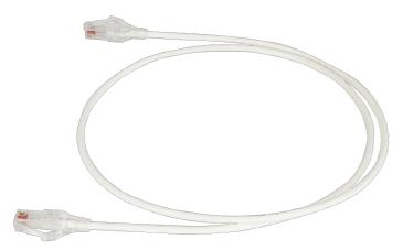
RDC 6 Modular Patch Cord, white, 3', reduced diameter, 28 AWG, cat6 channel four-pair UTP stranded PVC/CM.
