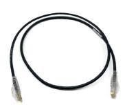
The RDC610 series of modular patch cords offer the reduced diameter of four pairs of 28AWG conductors, providing CAT6A channel performance for high density applications, when looking to reduce congestion or improve airflow through cabling pathways. Common applications include high-density cabling areas such as data centers, end-of-row (EoR) and top-of-rack (ToR) installations or areas such as telecom rooms and equipment rooms.
