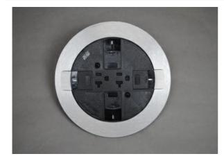
Kit comes complete with (1) prewired 20A duplex receptacle, (receptacle can be wired as a standard receptacle, or isolated ground), flange and slide holder, adapter ring to secure into the boxes, divider (RP-DIV), Wiremold CM Series open system adapters (unloaded), Ortronics Series II, and TracJack adapters. Modular jacks and A/V connectors sold separately.
