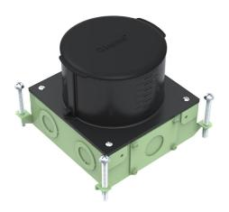
Rectangular dual service metal concrete floor box with a nonmetallic top that allows for concrete pours between 4" thick to 6" thick. Graduated markings on the inside and outside of the box indicating volume capacity, as well as the depth of concrete pour. Box accepts 2HUB to allow 2" conduit feeds (sold separately) while maintaining a 4" deep concrete pour. Box includes: (1) Reusable concrete cap (2) Removable knockout plates to allow the 2HUB to be attached.
