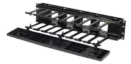
Single Sided Horizontal Managers are available in 1RU and 2RU sizes. The unique finger design protects cables from damage while the cover mounts with six hinge clips to allow the door to be opened one handed without becoming "unhinged". They are designed to mount on any 19" EIA style rack or cabinet.
