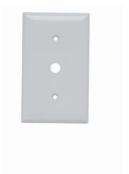
Single-Gang, Single telephone or cable outlet 13/32-inch hole. Strap mounted with adjustable yoke. One #340 yoke. Smooth thermoset. .
