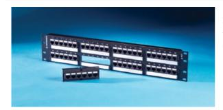
24- and 48-port TechChoice® patch panels are available in the traditional multi-port panel format with 6-port modules for Cat6 and Cat5e. Patch panel kits are also available to support individual keystone jacks. This panel is a Category 6 patch panel, 48-port, universal T568A/B wiring, six-port modular, 2 rack units.
