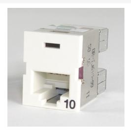
Clarity 10G TracJack, ETL tested as part of 100-meter 10 Gig channel solution. Front-loading and front removable. Universal T568A/B wiring label and tapered wiring towers simplify termination. Center tuned with synchronized reactance to Clarity 10G patch cords for optimum performance with minimized internal and alien crosstalk.
