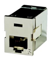
Clarity 6 Shielded, TracJack, ETL verified to TIA Category 6 component specification. Front-loading and front removable. New universal T568A/B wiring label and tapered wiring towers simplify termination. Center tuned to Clarity 6 Shielded patch cords for optimum performance.
