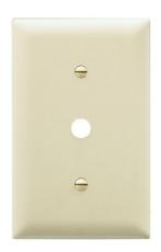
Single-Gang, Single telephone or cable outlet 13/32-inch hole. Strap mounted with adjustable yoke. One #340 yoke. Nylon Trademaster plate. .
