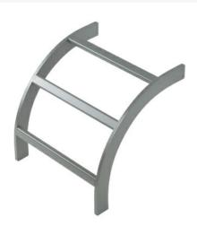
Radius curved runway permits smooth vertical to horizontal transitions. Stringers are 1-.5 in x .375 in steel tubes; cross slats are 1 in x .5 in x .125 in steel tubes. UL listed.
