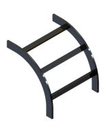
Radius curved runway permits smooth vertical to horizontal transitions. Stringers are 1-.5 in x .375 in steel tubes; cross slats are 1 in x .5 in x .125 in steel tubes. UL listed.
