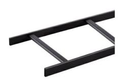
Universal Style Tubular Runway features 1 in x. 5 in tubular cross slats that are welded between  $.375 \times 1.5$  in high tensile tubular steel stringers. Cross slats feature rounded edges for cable protection. Standard length is 9ft 11 in, and widths from 6 in to 24 in. Available in rust-resistant, powder coated black finish only. UL listed.
