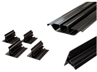
Consists of a 5' (1.524mm) length of divided base, 5' (1.524mm) length of mounting hinge rail and four (4) latching clips. Black, nonmetallic construction. Base width without Rail and Clips: 5" (127mm). Base width with Rail and Clips: 6 13/16" (173mm).
