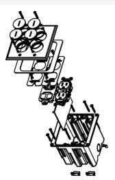
Wiremold WMFB2DRKS4N Series Dual-Gang Floor Box Assembly Part No. WMFB2DRKS4N
