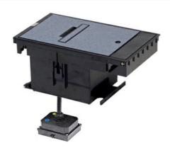
The gray Outdoor Ground Box cover assembly is prewired on a single circuit with [2] 20A weather resistant duplex receptacles. CAUTION: All ground box electrical circuits must be protected by a Ground Fault Circuit Interrupter upstream from the ground box.NOTE: Cover must be closed while in use. Use only molded plug and cord assemblies that are rated for outdoor use.NOTE: Maximum length of plug allowed at end of cord is 3" [76mm].
