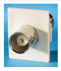
The TracJack, BNC Female to Female Adapter, Fog White Adapter Plate, has a single  $75\Omega$  BNC feedthrough connector, mounted at a  $180^\circ$  exit angle. This adapter panel is 1 unit high. TracJack modules offer flexabilty with structured cabling at the workstation or in furniture with a modular design and a wide variety of connectivity options. Inteligent engineering simplifies and speeds up moves, adds, and changes with a front removeable design. Compatible With: All TracJack faceplates
