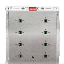
The InFusion Latching Relay is an integral component to Vantage's centralized lighting control system. It can be mounted in a main or secondary power enclosure and supports control of up to 8 loads with up to eight line feeds and up to 80 total amps of load.
