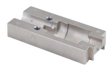
AFL compatible, Metal, Splice on Connector holders (60S), are specifically designed to fit the AFL 12S, 19S, 31S, 41S, 60S, 70S, and 90S model fusion splicers. Use this to hold the connectors inside the splicer when terminating Infinium splice-on connectors to ensure proper fusion splicing
