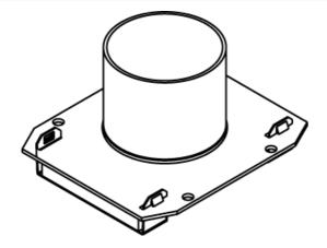
Two-gang 2" trade size conduit housing assembly. Used on 8AT Series devices. Covers two (2) of the three (3) gangs in the center compartment. Only for use with 8AT Series units.
