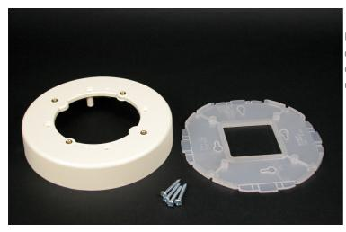
For hanging fixtures, smoke/fire alarms and other security devices with 3 1/2" (89mm) or 4 1/16" (103mm) mounting centers. 5 1/2" (140mm) diameter with open base. Not for use with fans.
