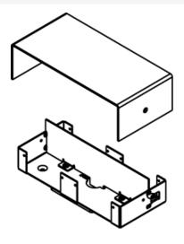
Double width housing for 241 Series Service Head. Barrier included (may not be needed for single service applications). Base has a 3/4" trade size KO for connection to FIT insert. Order two faceplates to complete service head assembly. NOTE: Assembled with scrub water gasket. For use on tile and carpte floors.
