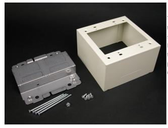
Two-gang, labor-saving, over-the-raceway device box. Cover has twistout on all four sides for 2400 Series Raceway. Accepts industry standard faceplates for electrical and communication devices. NOTE: Accepts NEMA double-gang standard faceplates. Certified to Canadian Safety Standards for sale in Canada. When ordering this product for Canada, add "C" to the beginning of the part number to denote Canadian versions, i.e. "CV2444" or "C2444-FW".
