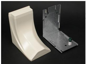
Eliminates need to offset 2400 Series Raceway when connecting with surface panel boxes. Has 3/4" and 1" concentric trade size KOs with 1" trade size KO elongated so adjustment from surface to center of bushing is 1" (25mm) minimum to 1 5/8" (41mm) maximum. Has twistouts for transition to 1500 and 2600 Pancake Raceways.
