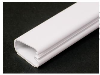
The Uniduct Nonmetallic Latching Raceway System is a one-piece, single channel design, ideally suited to route and protect fiber optic, UTP, and other low-voltage (50V or less) cables in an easy to install and aesthetically pleasing application. The 2800 and 2900 Fiber Optic (FO) fittings maintain a 1 1/4in (32mm) bend radius and are the perfect solution for even the most demanding cabling applications.
