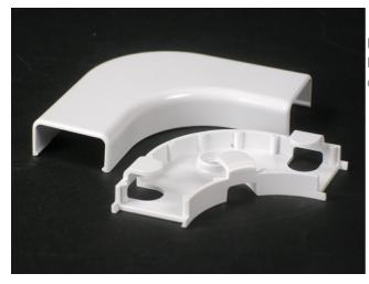
Makes right angle turns in 2800 Series Raceway on same surface. Maintains 1 1/4'' (32mm) bend radius when installing UTP and fiber optic cable.
