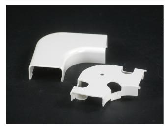
For right angle turns on same surface. Maintains 1 1/4'' (32mm) bend radius when installing UTP and fiber optic cable.
