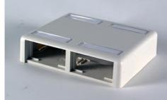
Ortronics Series II Surface Mount Outlet Boxes accept front-loading Series II modules and provide snap-on covers and snap-in label fields. Boxes are supplied with screws and double-sided adhesive tape for mounting onto almost any surface. Compatible with Wiremold 2700, 2800 and 2900 raceway series.
