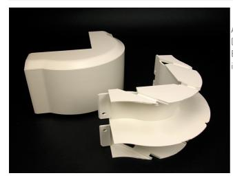
A 90 degree external corner with integral dividers to provide 2'' (51mm) cable bend radius for UTP and fiber optic installations. Each leg is 4 1/2'' (114mm). Ideal for lay-in or pull-through installations.
