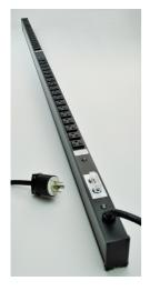
Two circuits with two 20A resettable circuit breakers. Thirty-six 20A outlets with T-slots, black housing. 12' (3.6m) cord. Length 70'' (1.8m).
