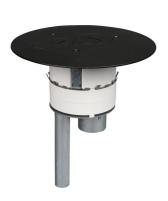
Complete with one-piece finish flange and conduit assembly. Conduit assembly consists of one 3/4inch trade size conduit and one 1 1/2inch trade size conduit. Finish cover flange provided with one 3/4inch trade size screw plug opening and one 1 1/2inch trade size screw plug opening. Covers available in painted black (BK), gray (GY), brass (BS), bronze (BZ), and brushed aluminum (AL). NOTE: Assembled with scrub water gasket. For use on tile, wood or carpet floors.
