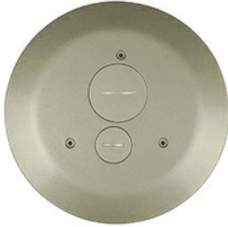
Complete with one 3/4" and one 1 1/2" trade size conduit adapters and closure plugs. Covers available in painted black (BK), gray (GY), brass (BS), nickel (NK), bronze (BZ), and forged brushed aluminum (AL). Use with the 4FFSTC15 insert to form a complete poke-thru assembly. NOTE: Assembled with scrub water gasket. For use on tile or carpet floors. 4FFATC Series Poke-Thru Devices require a 4" (102mm) diameter hole.
