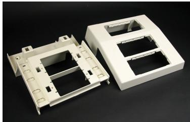
For mounting up to three power or communication devices at one location inline and offset with 5400 Series Raceway. For use with 5507 Series Faceplates, Ortronics TracJack and Series II Modules, Pass and Seymour Activate Series Inserts, Wiremold Open System Communication Modules. NOTE: CM-EPLA End Plates are required when using Wiremold communication modules. S2-EPL End Plates are required when using Orthonics Series II Inserts. To mount TracJack inserts, use 5507-4TJ or 5507-6TJ Faceplates.
