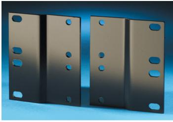
Ortronics® rack adapter kits allow 19″ equipment to be used on 23″ EIA racks. Includes #12-24 mounting hardware.
