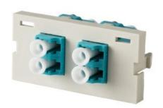
The Series II, Dual, Multimode, LC Duplex, Aqua Adapters (4-Fiber), Beige Adapter Plate, has two duplex adapters with 180° exit, and ceramic alignment sleeves. This adapter panel is 1 unit high. These adapter panels include dust caps, and offers two insests for optional icons (Not Included), to label each connector and indicate its purpose. Compatible With: Series-II Workstation Face Plates and Series-II Workstation Surface Mount Boxes. Wiremold raceway series 2700, 2800, and 2900
