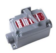
Double-Pole, Single Phase Switch in a NEMA 7 and 9 Enclosure for Hazardous Locations. Class I - Groups C, D Class II - Groups E, F, G. 30A, 600Vs. Slotted opening on enclosures allows for lock-out, tagout functionality.
