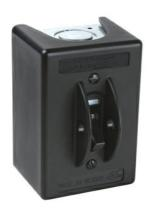
AC Manual Motor Controller, suitable as Motor Disconnect - 10KA @ 600VAC, 30A max. Class J Fuse.
