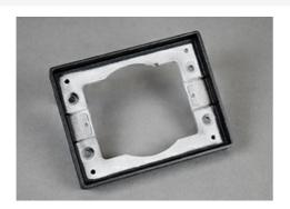
One-gang powder-coated aluminum tile flange, 4.5" x 3.5" (114mm x 89mm). For use on 880S1, 880M1, 880CS1-1, and 880M1-1 Floor Boxes. NOTE: UL Listed for tile, terrazzo, and carpet floors. Brass covers and flanges are not interchangeable with aluminum or nonmetallic covers and flanges. Nonmetallic covers are interchangeable with aluminum flanges.
