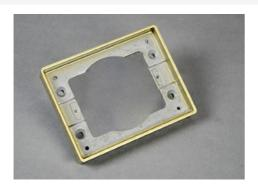
One-gang powder-coated aluminum tile flange, 4.5" x 3.5" (114mm x 89mm). For use on 880S1, 880M1, 880CS1-1, and 880M1-1 Floor Boxes. NOTE: UL Listed for tile, terrazzo, and carpet floors. Brass covers and flanges are not interchangeable with aluminum or nonmetallic covers and flanges. Nonmetallic covers are interchangeable with aluminum flanges.
