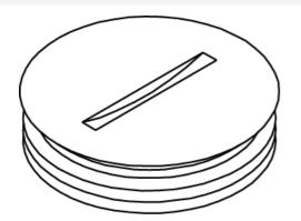
1" (25mm) diameter brass abandon plug. Thread size is pipe thread size.
