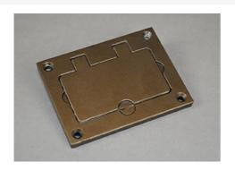
Brushed aluminum GFI cover plate, 3.290" x 4.310" [83.6mm x 109.5mm]. May be used with Wiremold CM Series adapters and Ortronics Connectivity Systems in conjunction with 817B, 827B, and 837B Flanges. Made in USA.
