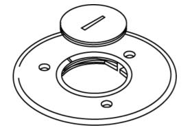
Brass communications or power cover plate with 2 1/4" (57mm) threaded opening for carpet. NOTE: For carpet or tile installations. All cover plates are furnished with gasket and three screws. The 895P Polycarbonate Series Cover Plates must be field modified for dual service.
