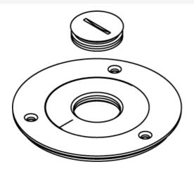
Brass cover plate with 1" (25mm) threaded opening for tile. NOTE: For carpet or tile installations. All cover plates are furnished with gasket and three screws. The 895P Polycarbonate Series Cover Plates must be field modified for dual service.
