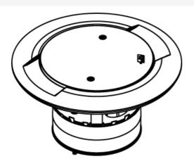
Complete plug assembly for abandoning an open 4" (102mm) diameter hole. Assembly includes intumescent fire-stop material to maintain the fire-classification of the floor, integral retainer ring to prevent the unit from pulling up through the floor, and a black diecast aluminum cover.
