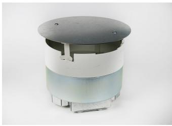
Complete abandonment plug assembly for 8" opening. Assembly includes intumescent fire stop material to maintain a 2 hour fire rating of the floor.
