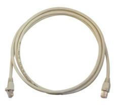
This component rated 500 MHz Cat 6a patch cable fully supports 10 Gigabit Ethernet up to 100 Meters. The snagless boot protects the tab from catching on other cables in a high density patch panel application. These pat
